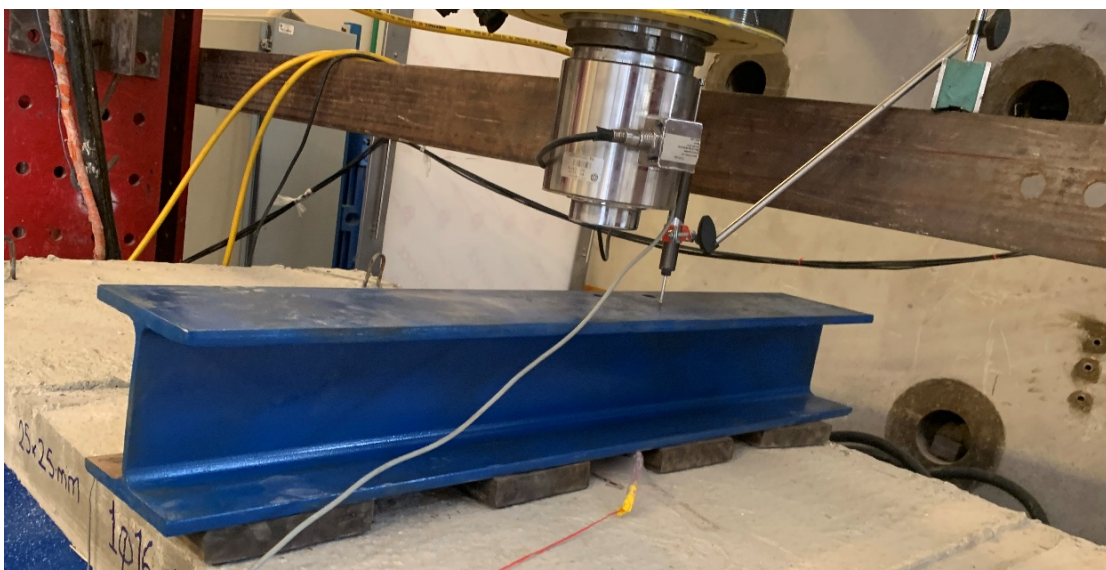
Figure 3.10 Loading beam and rubber pads
