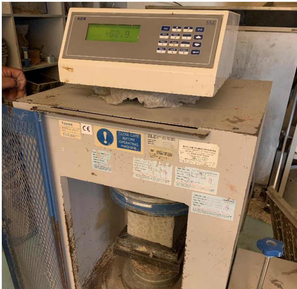
Figure 4.1 Concrete Cube Testing
