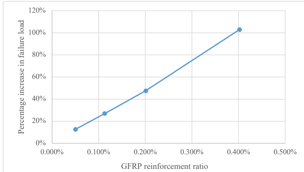
Figure 4.48 Percentage increase in failure load vs. GFRP reinforcement ratio
