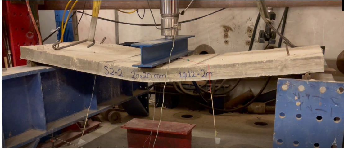
Figure 4.11 Series 2-2- Sample Failure
