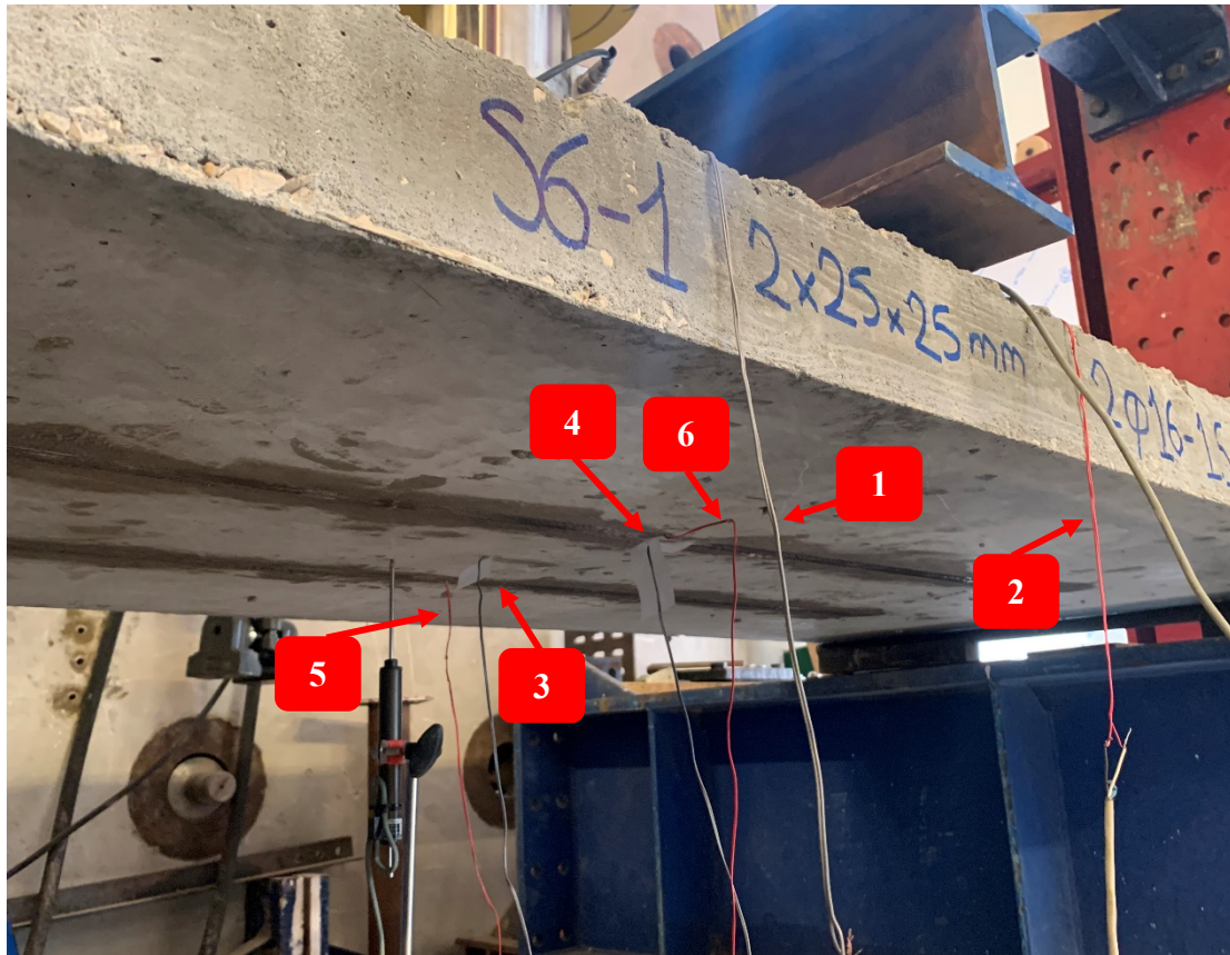
Figure 3.19 Location of Strain Gauges
